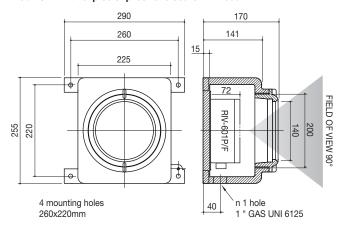
Note: In the model RIV-601P/FA the detector RIV-601P/F is to be mounted inside the explosionproof case by the customer during the installation phase, through the front window, over the steel plate provided on the bottom.
