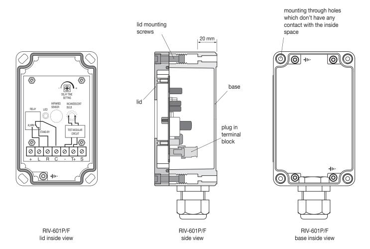
The enclosure base part has four mounting holes.
