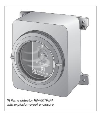
Normally the detector is installed vertically, centred on the area to be covered, so as the 90° cone field of view can be fully used. The ideal height is 0.7 the side of the square area.
