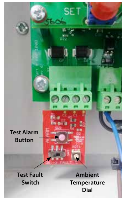
Figure 12: Analogue test board installed in control unit
