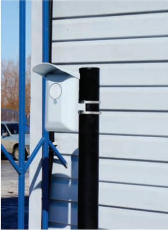
The principle of operation is based on the operation of two channels working on two different physical principles of detection: monostatic microwave and monostatic infrared.
