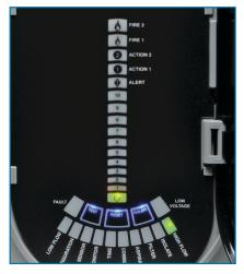
FAAST<sup>TM</sup> User Interface Display The User Interface consists of 5 Alarm levels – Alert, Action 1, Action 2, Fire 1, and Fire 2, 10 Particulate levels, 10 Bi-colour Flow and Fault graph.
