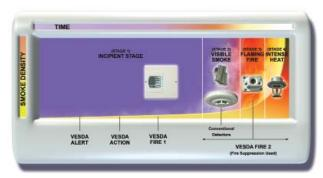
A VESDA smoke detector can be configured to detect a fire at the earliest stage. The multiple alarm levels can be configured to initiate an appropriate response at all stages of a fire.
