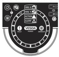
When the field service access door is open, the user has access to the RESET O DISABLE , Fire Test , AutoLearn and Instant Fault Finder functions. When the Instant Fault Finder function is activated, the Smoke Dial™ converts to a fault indicator, with the dial segment numbers corresponding to the faults listed below.
