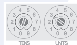
Figure 10: Decade address switches address 03 selected
